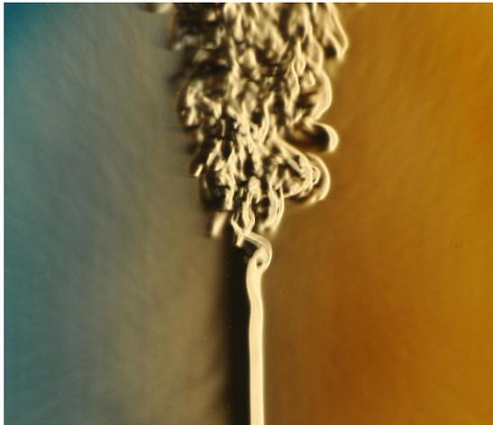
Figure 2.2: The plume of smoke from a candle flame transitions from laminar to turbulent flow [Set09].
