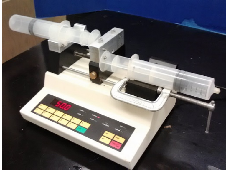
Figure 4.4: The Harvard Apparatus No. 55-2222 syringe pump was modified so that it could be used for simultaneous injection and suction. An aluminum syringe holder was added on the left end of the pump, allowing a second set of syringes to operate in the direction opposite to the manufacturer's design. An aluminum block was bolted to the pusher block allowing the plungers on the syringes, which normally just rest against the pusher block, to be bolted to it. The barrels of syringes on the right side of the pump were bolted to the aluminum blocks. The barrels of syringes on the left side of the pump were clamped to the syringe pump body. Together, these modifications allowed the syringe pump to draw fluid in addition to injecting it and operate in both directions.
