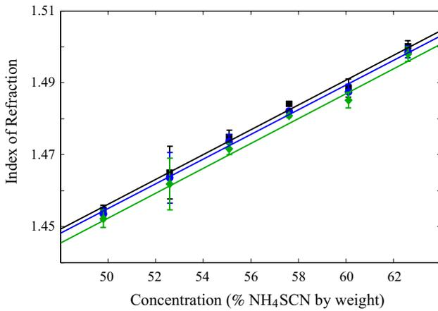
**Fig. 2** The index of refraction of NH<sub>4</sub>SCN solutions increases approximately linearly with concentration (% NH<sub>4</sub>SCN by weight) at fixed temperatures of 17 °C (black squares), 23 °C (blue circles), and 29 °C (green diamonds). Error bars indicate the sample standard deviation of the index of refraction at a given concentration and temperature
