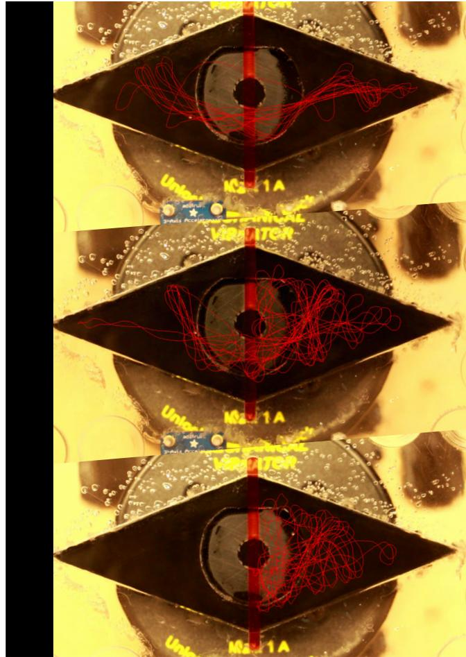
Figure 3.1: The the raw data from Trial 2. The red line in each image traces the path of the droplet for the duration of the trial. For each of the three barrier heights, the depth  $h$  of the oil above the barrier is shown, along with the fraction of droplets  $T$  that tunneled across the barrier.
