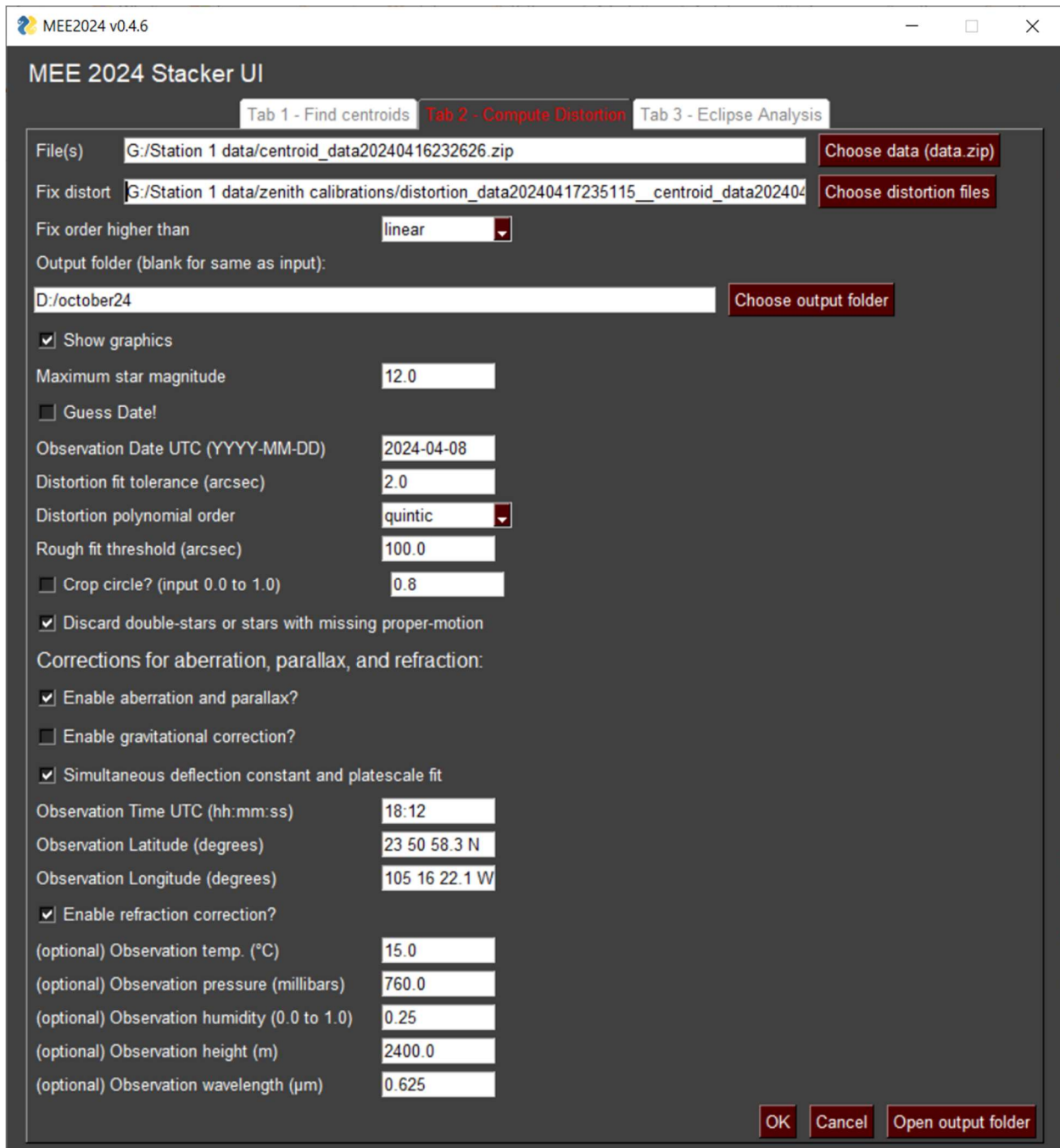
Figure 3: MEE2024 UI. Tab 2 is used for standard astrometry corrections (using AstroPy), characterizes the optical distortions of the telescope system, and applies the corrections derived from calibration frames to the eclipse frames. The output of Tab 1 is the input to Tab 2.
