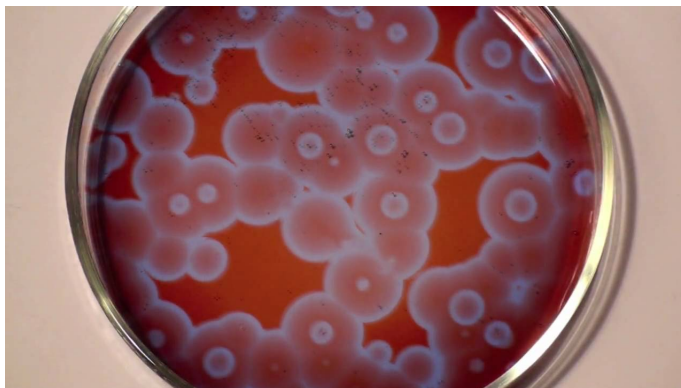
Figure 1: The Belousov Zhabotinsky reaction is performed in a Petri dish. Metal ions (cerium in this case) catalyze oxidation of the reductants by bromic acid in acidic water solution. The waves of oxidation are blue-gray [1].
