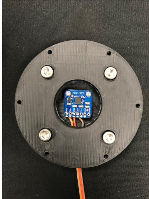
Figure 3.4: The ADXL326 triple-axis accelerometer, secured to the top of the vibration generator. Readings of acceleration are given in the z direction.
