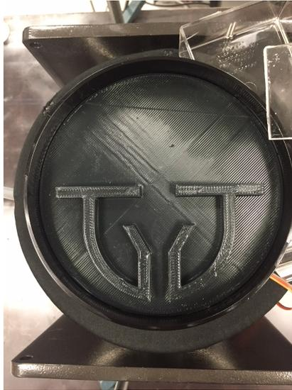
Figure 3.3: Our fluid bath setup without any silicone oil in it. Mounted in the bath is the 3D printed disk with the droplet launcher being the Y-shaped structure that opens toward the slit. The impact parameter of this particular setup is zero. The Plexiglas piece in the top right corner is the end of the ramp that directs the newly produced droplets onto the bath.
