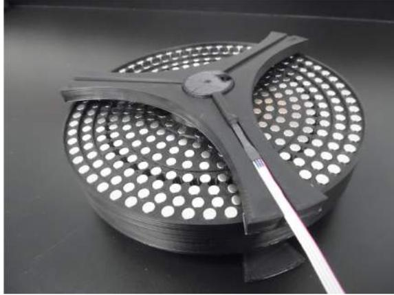
Figure 3.4: We measured the magnetic field at different distances from the center for Setup-3 using a gaussmeter and a few tools that we custom 3D-printed for positioning the magnetic field probe accurately.
