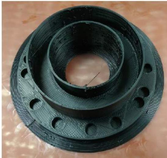
Figure C.1: A 3D print was made with magnet slots of varying radii, starting from 3 mm, stopping at 3.5 mm, and going up by  $(1/32)$  mm with each slot.
