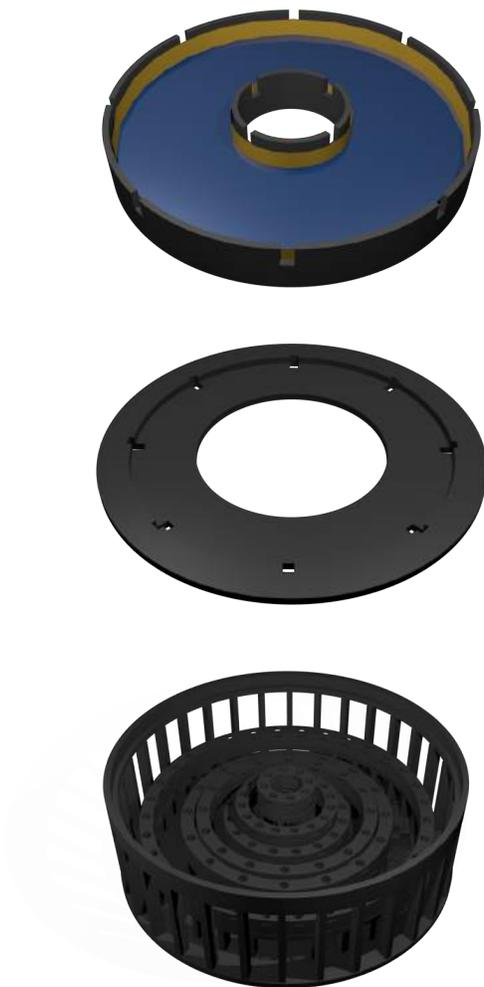
Figure 3.9: An assembly drawing of Setup-1. The magnet tray is a complex part with removeable rings of magnets. The water cell sits at the top as usual.
