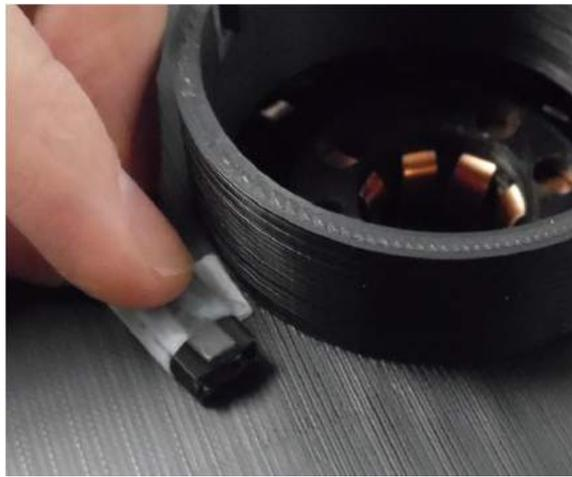
Figure 3.14: We measured the magnetic field at different distances from the center for Setup-1 using a caliper and a gauss meter. The gauss meter was carefully taped to a plastic piece of width 4.5 mm, almost the 5 mm for the water level, and placed on top of the water cell's floor for measuring.
