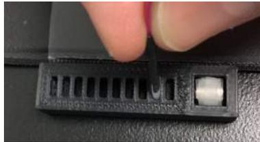
Figure B.5: The slots were just a little bit too big, so we put tape around the probe and magnet in order for them to fit perfectly.
