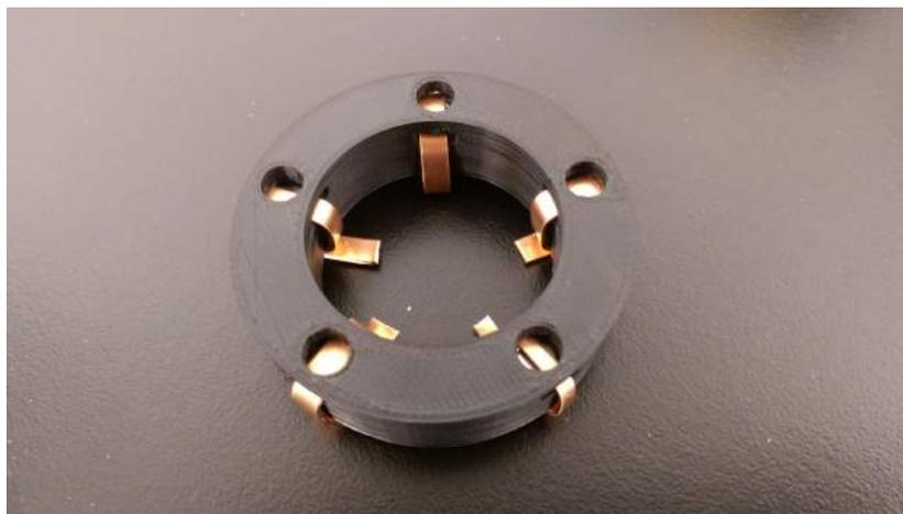
Figure 3.10: A test magnet ring with cylindrical slots for five magnets. The ring also has flat slots for copper shim stock to go through and hold the magnets in place. In case the magnets get stuck, there are small holes on the opposite side for pushing the magnets out with a thin tool. The magnets were inserted with the north (N) pole directed vertically *up*.
