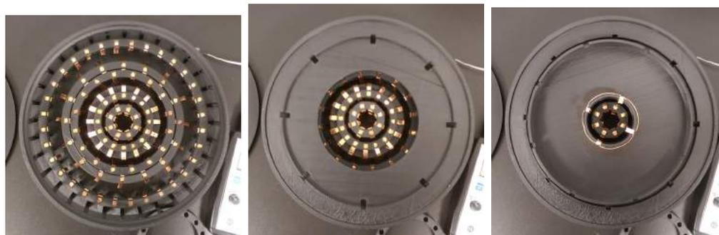
(a) Magnets uncovered.      (b) Magnets covered.      (c) Water cell on top.
