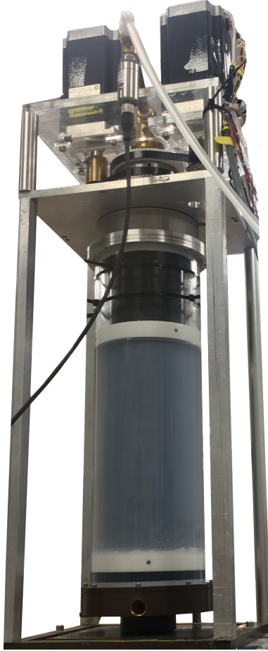
Figure 3.1: The Taylor-Couette apparatus is surrounded by its metal bracing. Mounted on top are the stepper motors that move the inner and outer cylinder. Through the outer cylinder, the rheoscopic fluid, white plastic rings, and black inner cylinder are visible. The tubing running to the right connects to the perturbation system, while the wire running to the left is connected to a pressure transducer. Not pictured is a USB camera which records images of the test section.
