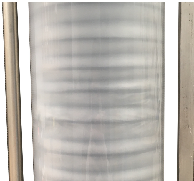
Figure 3.3: The Taylor-Couette system's Taylor vortices are easily visible when the rheoscopic shaving cream and water mixture is used to visualize the flows. Just as other rheoscopic fluids have shown, this Taylor-Couette flow produces bands in its lower Reynolds number and less spatiotemporally complex states. This shows that the shaving cream and water mixture is a viable method for flow visualization.
