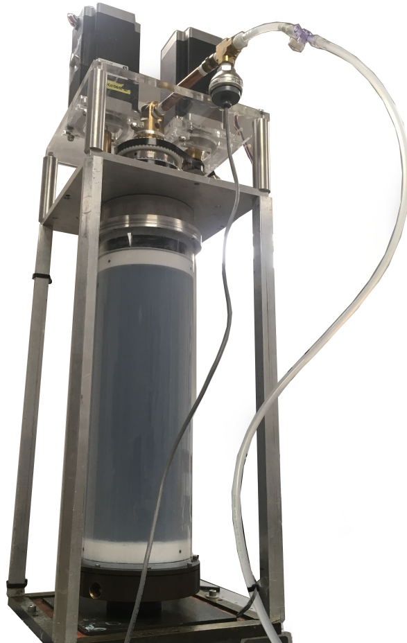
Figure 3.1: Within the outer cylinder, the inner cylinder can be seen though clouded by the shaving cream and water mixture. On top of the Taylor-Couette system's bracings are the stepper motors and timing pulley system. The tubing that can be seen running from the top of the system is connected to the perturbation system.
