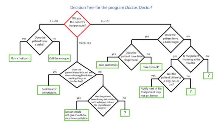
Each box is called a <u>node</u>. The top red node is called the <u>root node</u>; it is where the diagnosis begins. The green nodes at the bottom are called <u>leaf nodes</u>; they are where the final diagnosis can be found. Note that there are some missing leaves in the written rules. These are specified by "?" in the above tree. In these cases, it is assumed the doctor does not have a diagnosis; the program should let the user know this.
