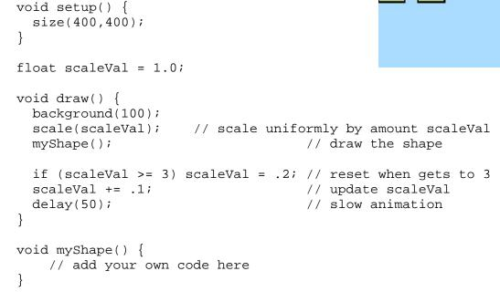
2. The Scale Transformation: Look up the **scale** transformation in the Processing reference. In the above code, the scale(scaleVal) scales the object *uniformly* in all directions by an amount scaleVal relative to the origin:
