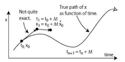
Euler's method is the simplest method for approximating differential equations. A much better approximation is called the *Midpoint* or *Runge Kutta Method* given by
