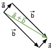
Figure 1.4: The same total displacement vector is found by summing  $\vec{a} + \vec{b}$  and  $\vec{b} + \vec{a}$ .
